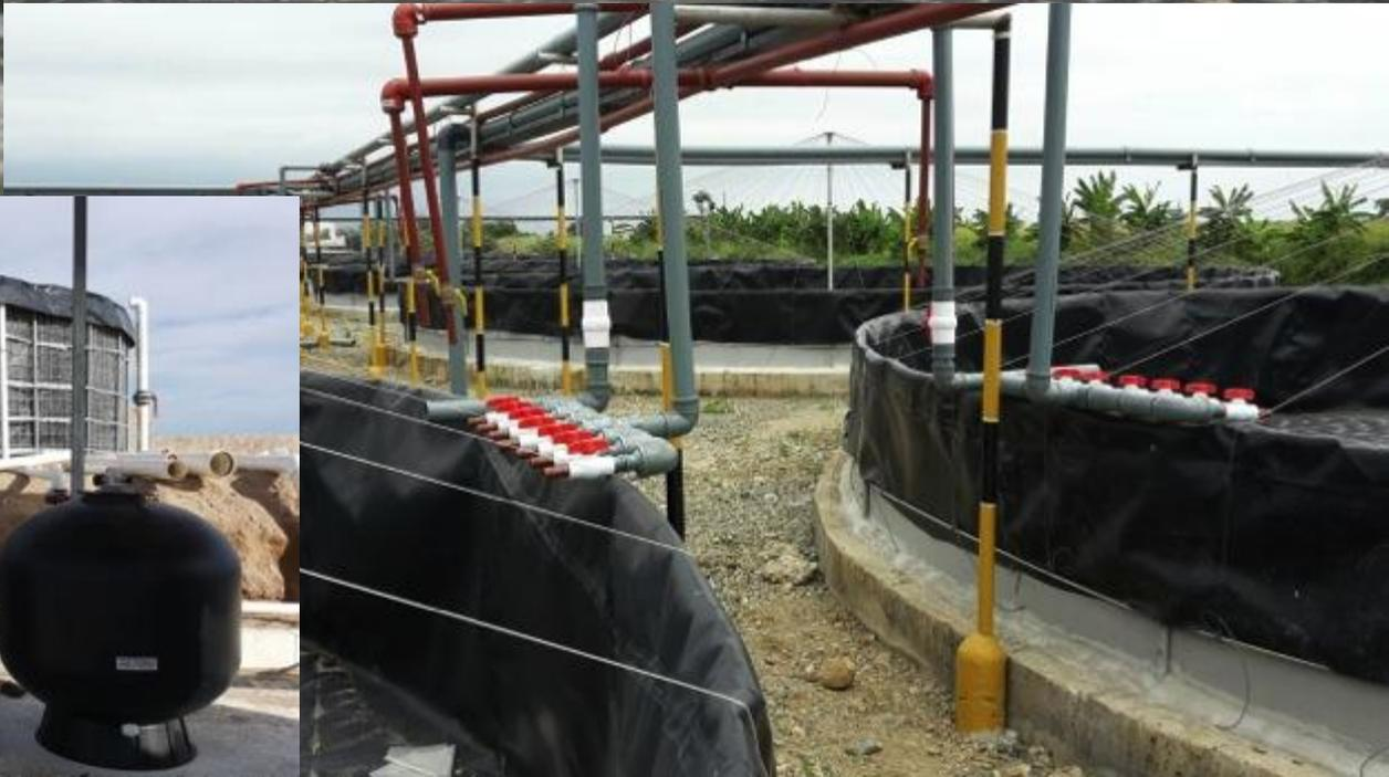
Reservoir: chlorine treated => probiotics => sand filtered => fill nursery raceway
